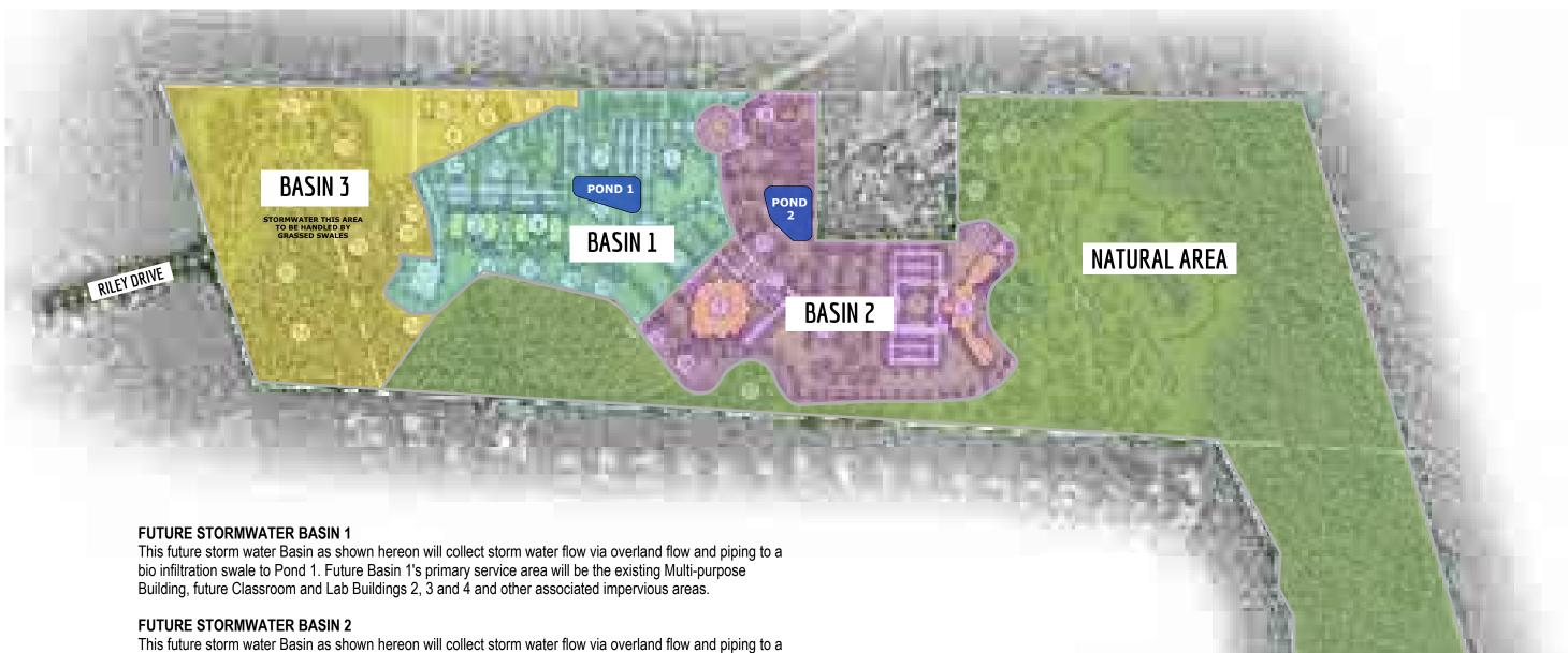
This future storm water Basin as shown hereon will collect storm water flow via overland flow and piping to a bio infiltration swale to Pond 2. Basin 2's primary service area will include the Eco Training Center and the ECO Tourism Hospitality Training Center buildings five and six respectively.
